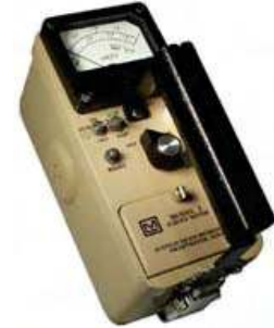
Figure 2. General Purpose Survey Meter
